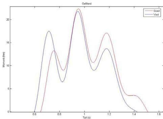
**Figure 1:** Graph of the 'reactive impact'. The red line is the Xco-Trainer, and the blue line the solid weight. The reactive impact is visible as the third peak.<sup>5</sup>
